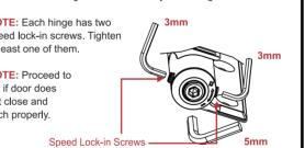
speed, latch speed, and closing tension reciprocally until slamming stops and door latches properly. **ADJUSTMENTS** • Door Slams: Reduce (-) swing speed or
