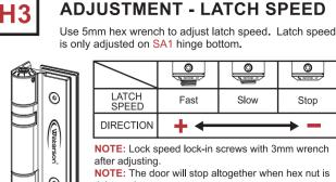
NOTE: Lock speed lock-in screws with 3mm wrench NOTE: The door will stop altogether when hex nut is tiahtened.
