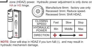
CAUTION: Hydraulic mechanism operates best from 0-120°. Opening beyond 120° will damage hinge and violate warr
