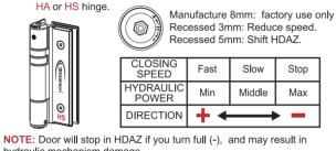
CAUTION: Hydraulic mechanism operates best from 0-120°. Opening beyond 120° will damage hinge and violate warran
