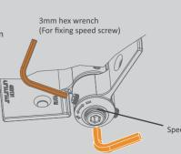
5 mm hex wrench (Speed screw: for adjusting closing speed)
